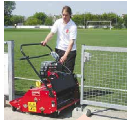
The width of the Verti-Top WB can be narrowed to 87cm enabling it to pass through small passways.
