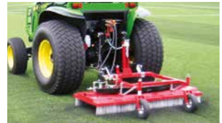
The 5 counter rotating brushes turn at high speed.
