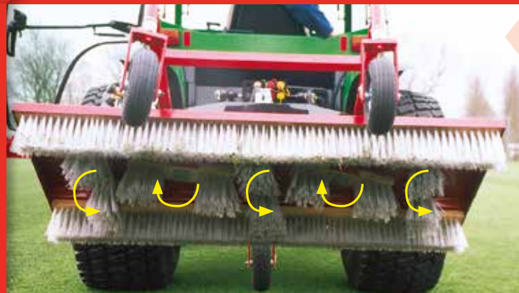
The 5 counter rotating brushes turn at high speed.
