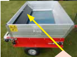
The Dry-sand plate ensures extra accurate spreading.
