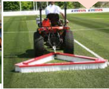
Model 240 has a large working width of 2.4m
