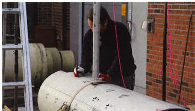
▲ Impact testing at Flowtite Technology laboratory in Norway.
