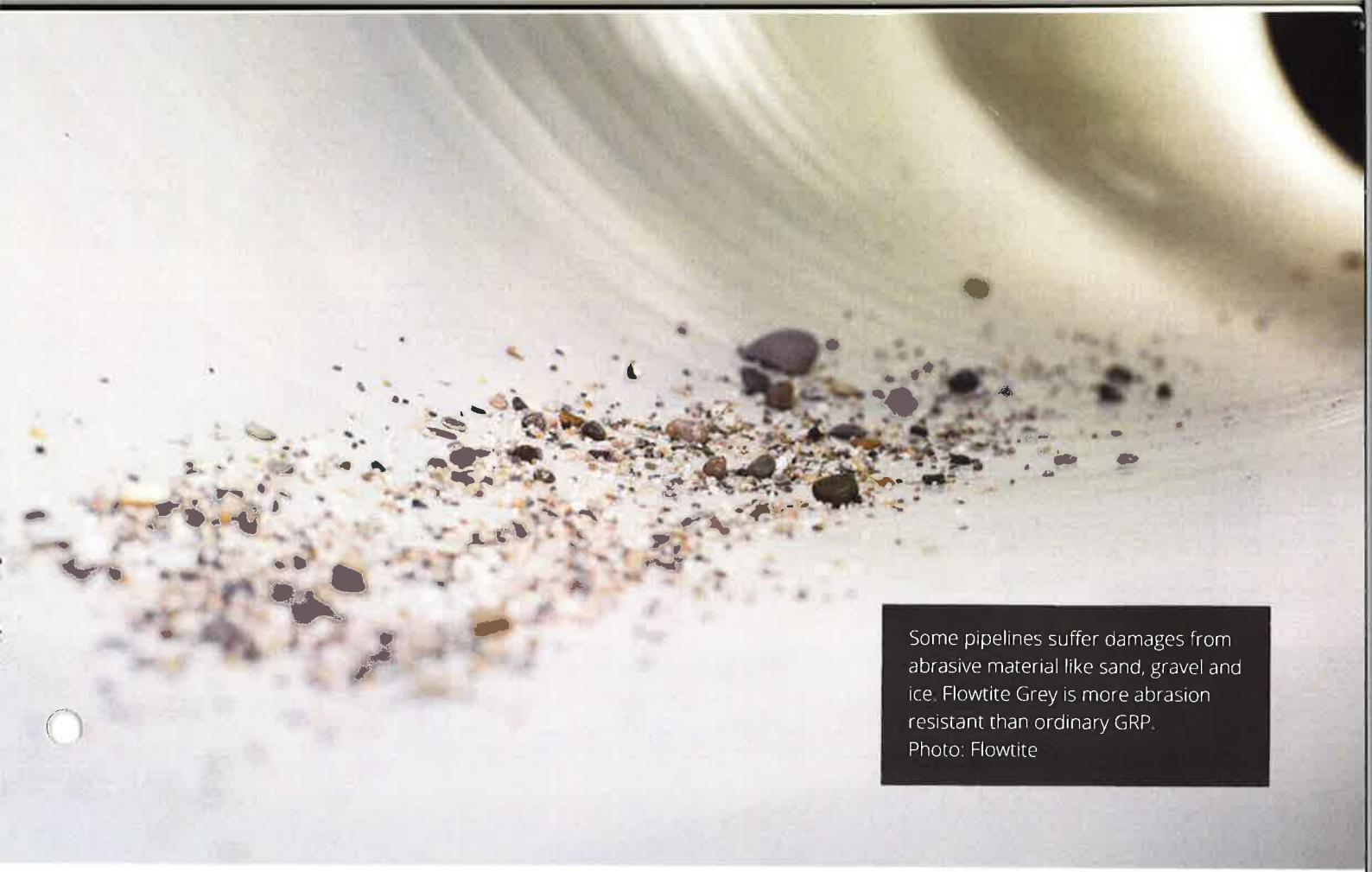
Some pipelines suffer damages from abrasive material like sand, gravel and ice. Flowtite Grey is more abrasion resistant than ordinary GRP.
