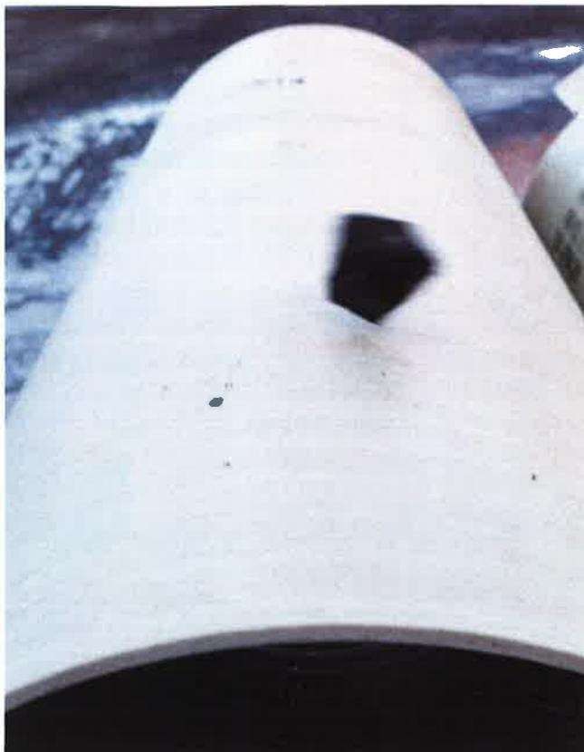
Impact resistance is the pipes' ability to resist impact. Impact resistance is typically measured by falling mass testing on empty and/or water-filled pipes. Impacted pipes are then inspected for damage and additionally, pressure tested to ensure water-tightness after impact.
